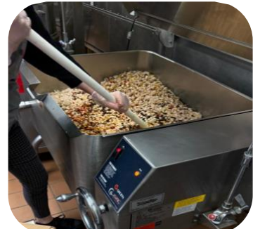
Tilt skillets can tilt to safely transfer products and cook large batches of scratch items like soup, raw meat, or chili.
