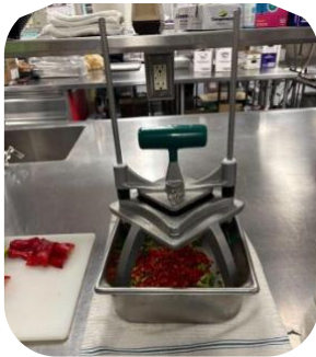
A countertop dicer dices produce in uniform size.
