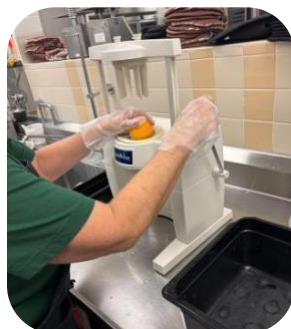
A sectionizer cuts produce into uniform wedges or slices, adding visual appeal.
