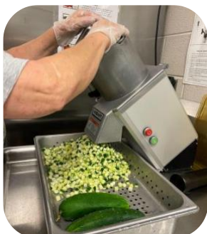
A continuous feeder cuts produce in uniform size.
