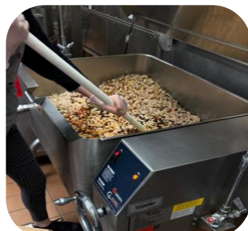
Tilt skillets can tilt to safely transfer products and cook large batches of scratch items like soup, raw meat, or chili.
